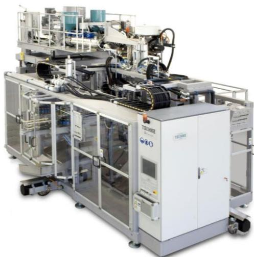
ADV2-700 is a full electric-mechatronic modular shuttle machine, which includes the most advanced technologic solutions on the market. With its double and four shuttle configurations, it is flexible and perfectly suitable for the end users and converters who look for a machine with medium to high production capacities and adaptability in terms of production. Its 700 mm stroke allows to produce containers from 60 ml (neck to neck) in 10+10 cavities to 5 L in 2+2 cavities, up to 6 layers.
